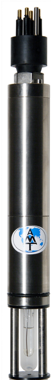
fig.: pH-combined electrode for deep sea use
